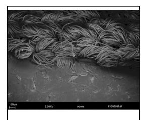
Figure 18. SEM image of ultrasonic welded knitted textile sample Author's own 2012
