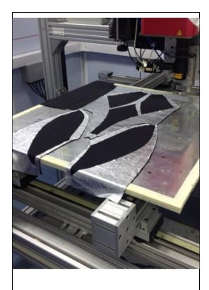
Figure 15. Preparation of flat panels for laser treatment at TWI
